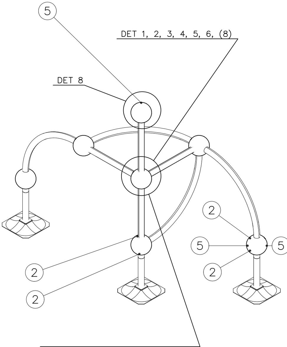
DO NOT TIGHTEN THE JOINTS UNTIL THE STRUCTURE IS COMPLETE.
