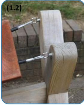
**2. Locate M8x80mm eye bolts** through pre drilled holes using flat washers on both sides of the timber to prevent the fixing pulling into the timber. Secure in place with **M8 nyloc nuts**, cover 4 holes in ends using **4x30mm caps (1.3)**
