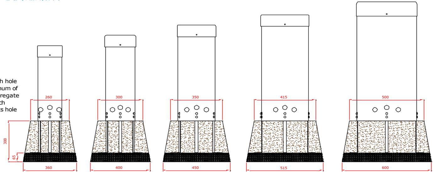
Foundations should not present a hazard. These foundations are recommended as a guide, for more information on foundation details for various surface see Part 7 of BS EN 1176.
